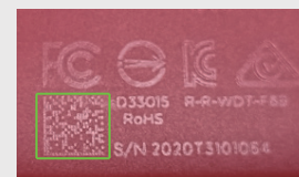
Laser engraved code for a solid state drive housing with very low contrast
