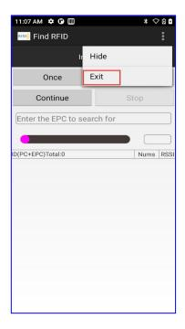
Implementation principle of development: call our uhf. Continuous card finding method in jar, List <EPC> epcList = mDevice.getTagIDs(); There is signal strength in the returned epclist, and the signal intensity of the label is updated in real time, which can be realized according to the signal intensity.
