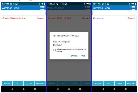
After a successful Bluetooth connection, the current connection status will be displayed in the upper left corner. When the client software exits, the device connection status is disconnected, and when the APP exits, the client software will exit the APP or the client program abnormally. Please disconnect the exit program and open it and connect again.
