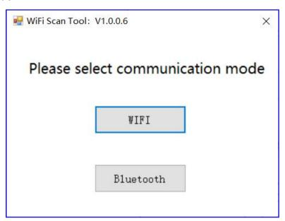
Whether choosing Bluetooth or WIFI, the corresponding IP / MAC address and QR code will be displayed for the device to scan the code connection;
