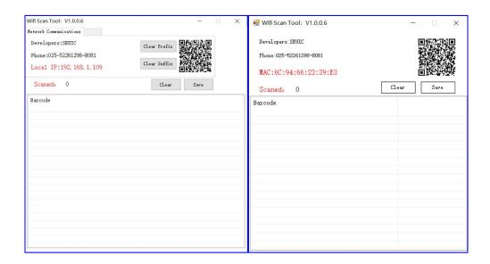
The received data will be displayed on the interface, and you can also click the text box / EXCEL table to transfer the data to the focus. After scanning the data, you can also directly click the save data button to save the data locally.
